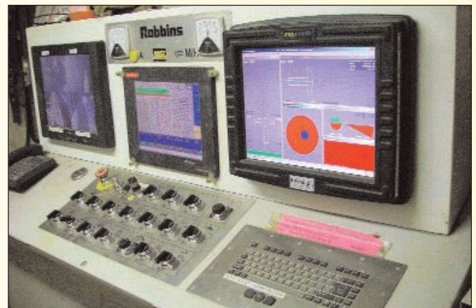
Figure 3.3.1 PPS guidance system total station bracket and computer in the TBM control cabin.
