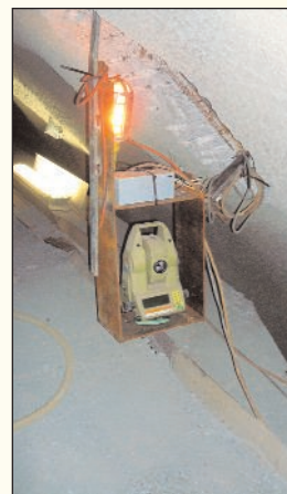
Figure 3.3.1 PPS guidance system total station bracket and computer in the TBM control cabin.
